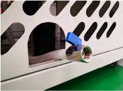
vacuum /water draining valve
